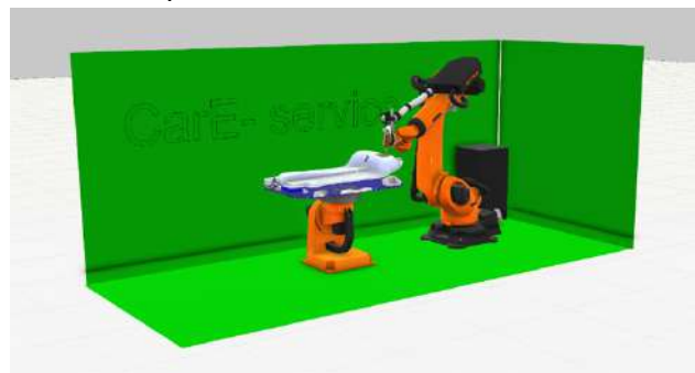
Side view of module. Robot perform unscrewing
